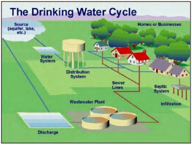
**Figure 8-3. Drinking water cycle** (Diagram by University of Florida IFAS Extension)
