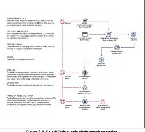
Figure 3-9. SolarWinds supply chain attack operation (Diagram by Microsoft)
