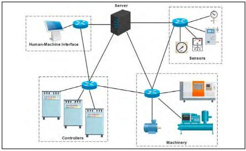
Figure 3-2. Typical OT industrial systems network architecture (Diagram by Applied Sciences)
