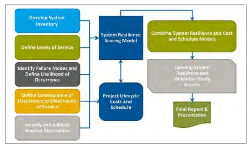
Figure 8-4. Process for the NCR water system study (Diagram by Black & Veatch)
