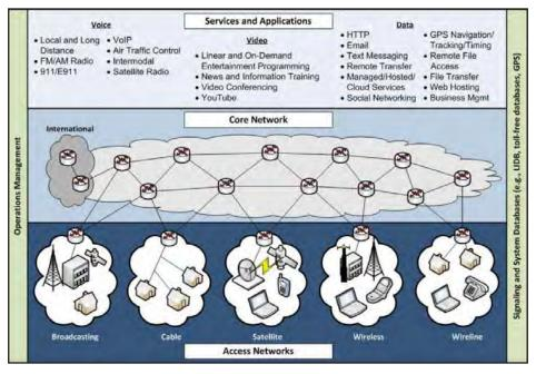
Figure 9-1. Communications sector architecture model (Diagram by Department of Homeland Security)
